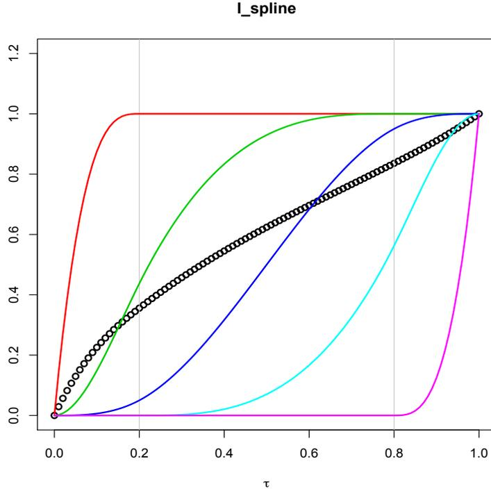
Figure 3: An example of the integrated spline (I-spline). The I-splines are defined on  $[0, 1]$  of order  $h=3$  and associated with interior knots 0.2, 0.8. Each I-spline is piecewise cubic, and a monotonic curve is obtained by the linear combination of these  $M=5$  splines with nonnegative coefficients  $(1.2, 2, 1.2, 1.2, 0.4)/6$ . The I-spline functions ensure non-crossing quantiles with both flexibility and constrains at different percentiles.
